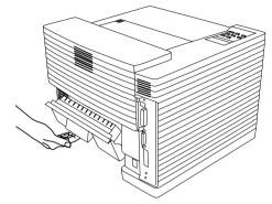
Carefully remove the paper from the Transfer Drum.
